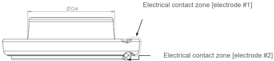
A  $5 \Omega$  max contact resistance is recommended for appropriate electrical connection.
